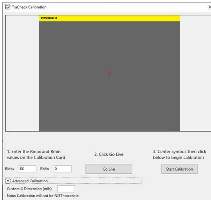
Use the Advanced Calibration option only if you use a non-NIST traceable calibration symbol. This option allows you to enter the Custom X-Dimension (mils) value of the barcode that you use to calibrate the unit. The calibration process uses the Custom X-Dimension (mils) value to calibrate dimension measurements.
