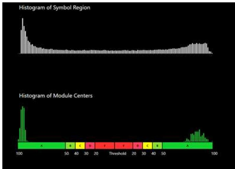
The horizontal axis on the **Histogram** represents the brightness level with the dark elements on the left side and the bright elements on the right side. As the element's brightness increases, the **Histogram** displays the element farther to the right of the **Histogram**. The height of each bar represents the number of elements with the same brightness associated with the elements' positions on the horizontal axis.
