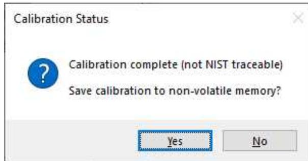
If you perform a successful calibration with a non NIST-traceable calibration symbol, no calibration date is recorded on the reports or displayed on the Main tab in the TruCheck window. Instead, The message reads "Calibration Complete (not NIST-traceable)".
