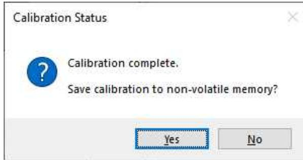
When you perform a successful calibration with a supported NIST-traceable calibration symbol, a calibration time date stamp appears on the bottom of the TruCheck window and is printed in the header of the report. For the list of NIST-traceable calibration symbols see the step list below.
